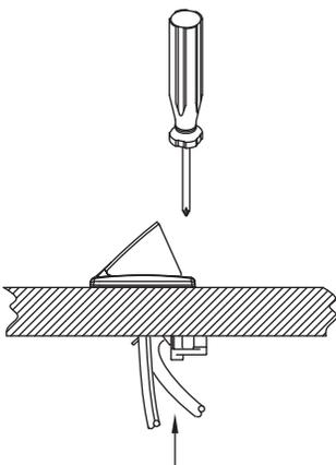
**Note:** In a conduit application, conduit should be supported according to local code. When managing conduit and cabling exiting the unit, ensure there is adequate slack to allow unit to open properly
