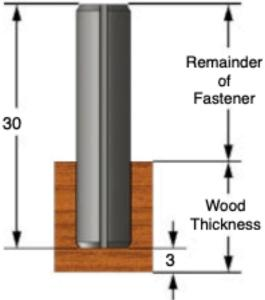
Plunge Cut: Z -10.5 | Slot: X 32 | Retract: Z 10.5 (Allowable depth range is -10.5 to -10.85)
