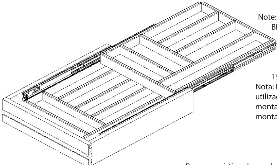
Note: The wood tiered drawer is designed to use either Blumotion 562F533-01B under mount slides or Grass Elite 7523-19/550/533 under mount slides.
