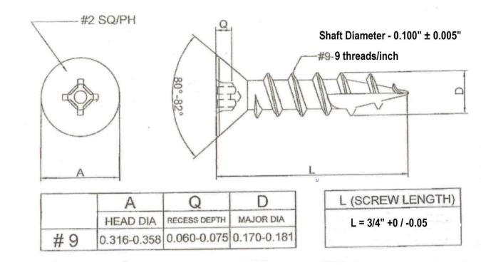
FLAT HEAD QUADREX WOOD SCREW TYPE-17 COARSE
