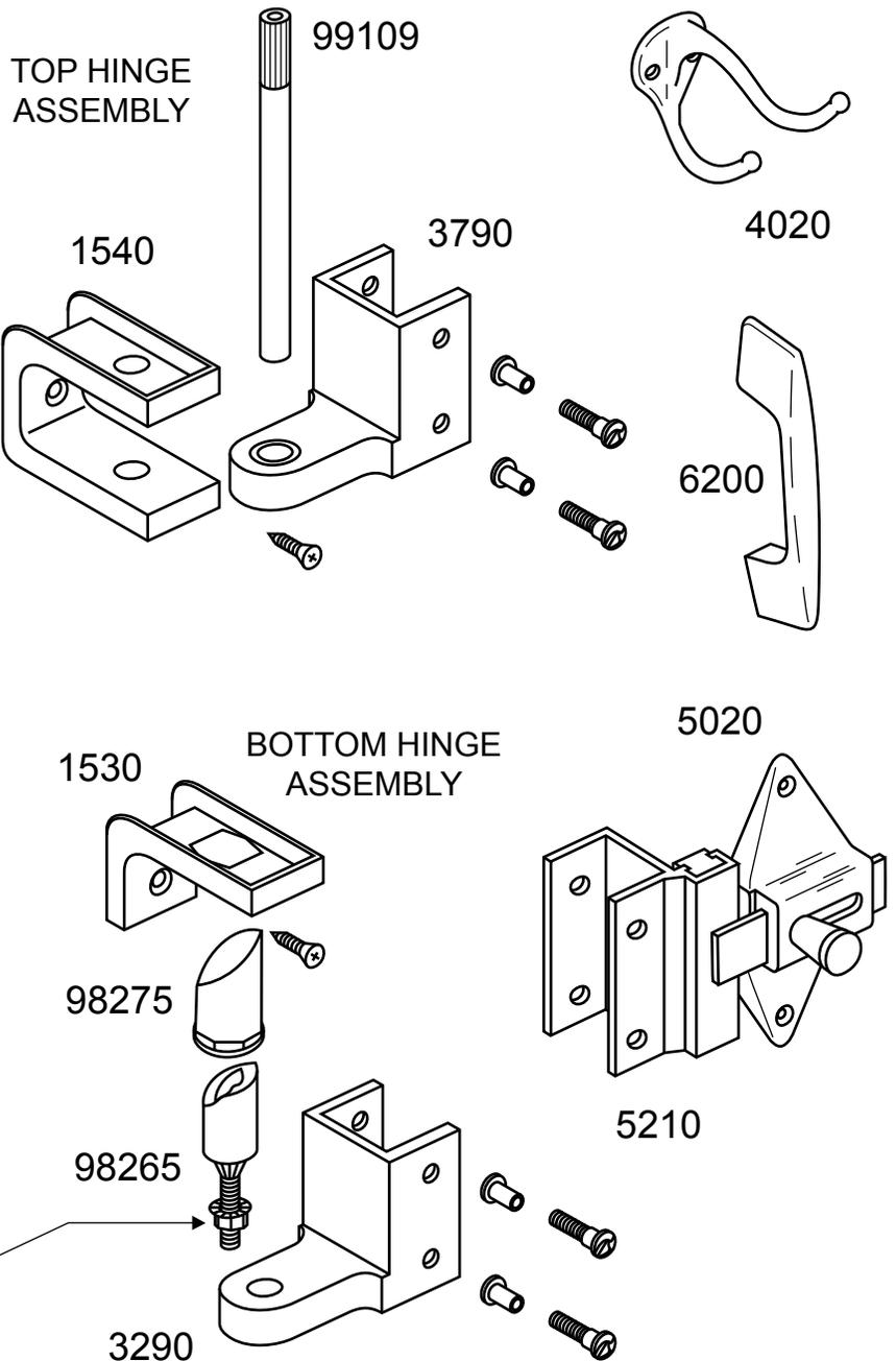
NOTE: adjust door to desired position and tighten nut.
