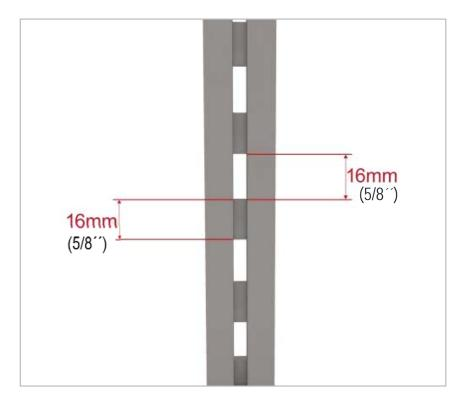
All slotted profiles must be oriented in the same direction during installation and should only be cut from the top. This ensures that all slots will be at the same height so drawers and shelves are evenly mounted.
